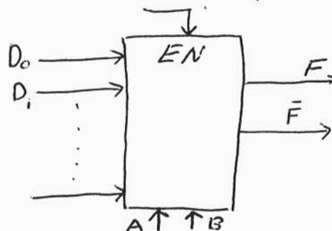
$D_0 \dots$  are the input "data" lines, 4 or 8 or 16 etc
