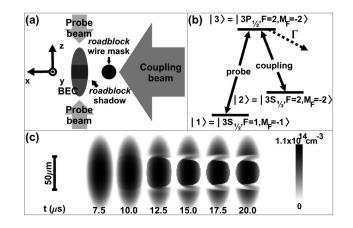
FIG. 1. Defect creation. (a) Double light-roadblock setup. (b) Energy level diagram. (c) Density plots of  $|1\rangle$  atoms from 2D simulations of defect creation using a 60  $\mu$ m wire mask; initially, the BEC has  $4.0 \times 10^6$  atoms. Light pulse intensities and durations are as in the experiment.
