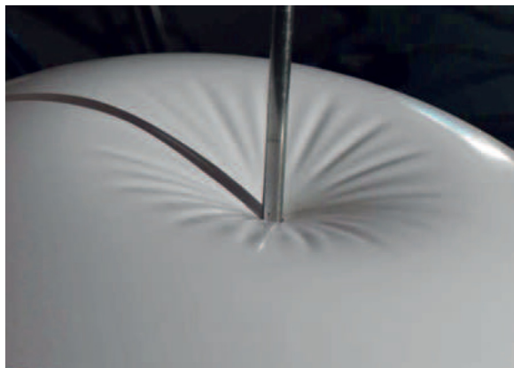
Fig. 16 Buckling of an inflated rubber ball subject to a cylindrical indenter (Reproduced with permission from Vella et al. [18]. Copyright 2015 by IOPscience.)
