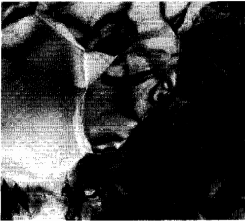
Fig. 4. Three examples of microcracks observed at twin terminations in the \text{Al}_2\text{O}_3/\text{ZrO}_2 interface.
