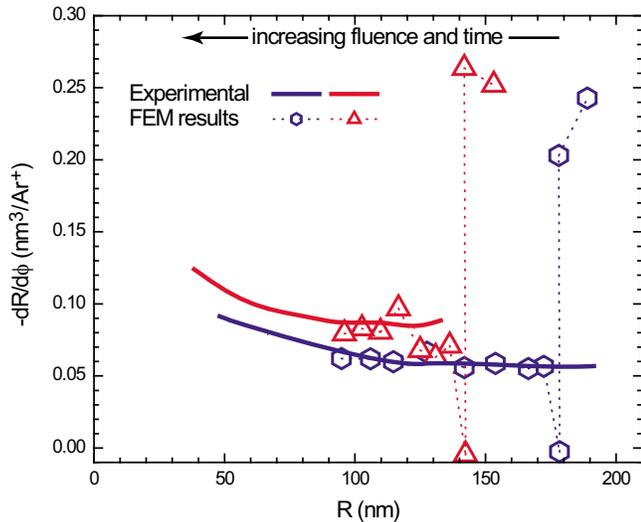
FIG. 6. (Color online) Nanopore closing rates  $-dR/d\phi$  vs instantaneous pore radius  $R$  for *a*-Si pores under  $0.24 \text{ Ar}^+ \text{ nm}^{-2} \text{ s}^{-1}$ . Experimental data are smoothed.
