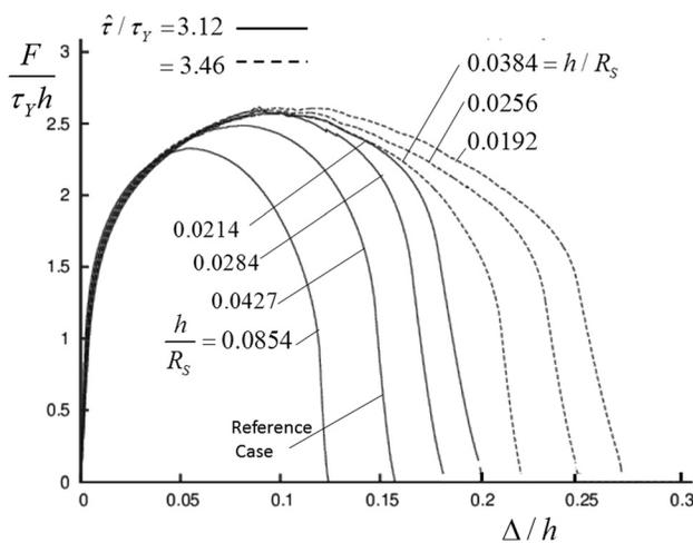
**Fig. 5 The role of  $h/R_S = \pi(1-\nu^2)h\tau_Y^2/(E\Gamma_0)$  on the normalized force–displacement relation for cropping for two values of  $\hat{\tau}/\tau_Y$  and with  $N = 0.185$  and  $\tau_Y/E = 0.000785$ . With all the other dimensional parameters fixed, each set of curves (for a given  $\hat{\tau}/\tau_Y$ ) can be interpreted as either the effect of varying  $\Gamma_0$  (with  $h$  fixed) or varying  $h$  (with  $\Gamma_0$  fixed). Cases 1, 11, 12, 13, 14, 15, and 16.**
