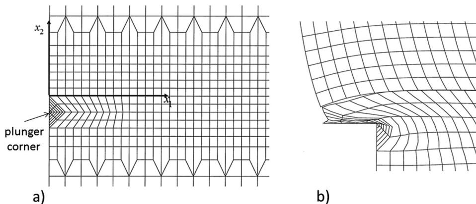
**Fig. 12** (a) Undeformed mesh for simulation with a gap  $d = 2D_0$ . (b) Deformed mesh with gap in the vicinity of the plunger corner for case 19 at  $\Delta/h = 0.108$ .
