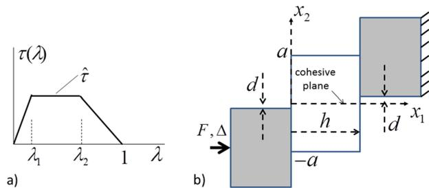
**Fig. 3** (a) The cohesive traction–displacement relation in shear. (b) The undeformed geometry of the numerical model showing the reference coordinates. The cohesive plane in the undeformed state lies along the  $x_1$  axis. The bottom surface along  $x_2 = -a$  is constrained to undergo frictionless sliding with zero vertical displacement. The upper surface along  $x_2 = a$  is traction-free. Sliding is suppressed at the contact surfaces between the rigid tools and the metal block.
