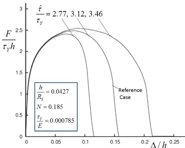
**Fig. 8** The role of the normalized shear strength in the cohesive zone  $\hat{\tau}/\tau_Y$  on the normalized force–displacement curve with the other dimensionless parameters held fixed. Cases 1, 10, and 11.
