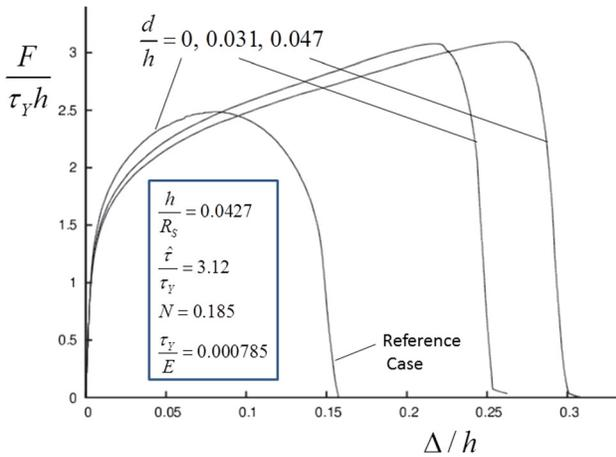
**Fig. 13** The role of a gap between the tool corners and the cohesive plane  $d/h$  on the normalized force–displacement curves with the other dimensionless parameters held fixed and equal to those of the reference case. Cases: 1, 19, and 20.
