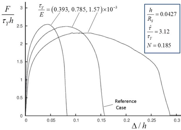
**Fig. 10** The role of  $\tau_Y/E$  on the normalized force–displacement curves with the other dimensionless parameters held fixed. As discussed in the text, the specific cropping work with the normalization  $\Gamma_{\text{CROP}}/\Gamma_0$  is only weakly dependent on  $\tau_Y/E$  with the other dimensionless parameters held fixed. Cases: 1, 2, and 3.
