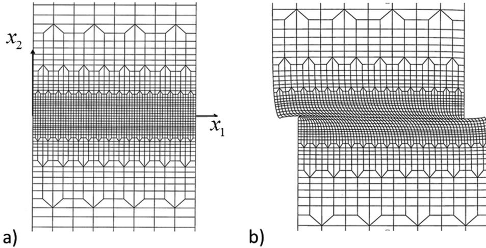
**Fig. 4 (a) The mesh in the undeformed state. The cohesive plane lies along the  $x_1$  axis. (b) The deformed mesh for the reference case (case 1) at  $\Delta/h = 0.136$ .**
