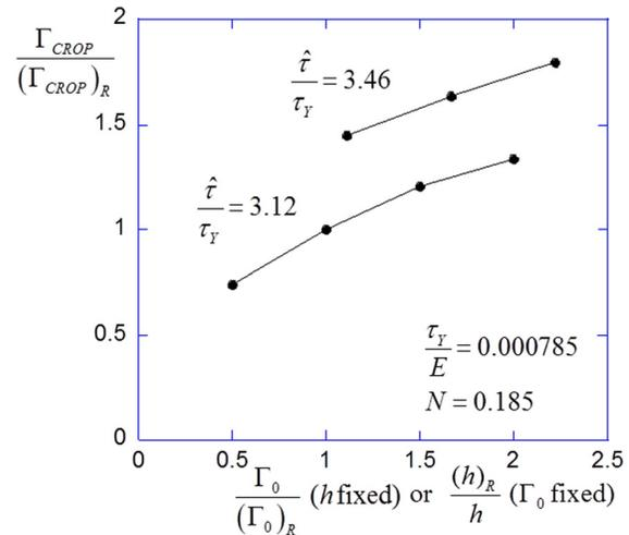
**Fig. 6 The dependence of the specific cropping work  $\Gamma_{CROP}$  on the microscopic specific work of fracture  $\Gamma_0$  for plates of the same thickness. Equivalently, the dependence of the specific cropping work  $\Gamma_{CROP}$  on inverse thickness  $1/h$  for plates with fixed material properties. The normalizing quantities denoted by the subscript  $R$  refer to reference case 1. The points plotted are cases 1, 11, 12, 13, 14, 15, and 16.**
