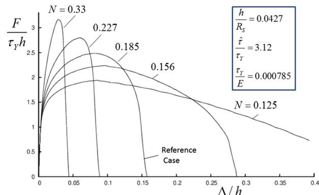
**Fig. 9** The role of the strain hardening exponent on the normalized force–displacement curves with the other dimensionless parameters held fixed. Cases 1, 4, 5, 6, and 7.
