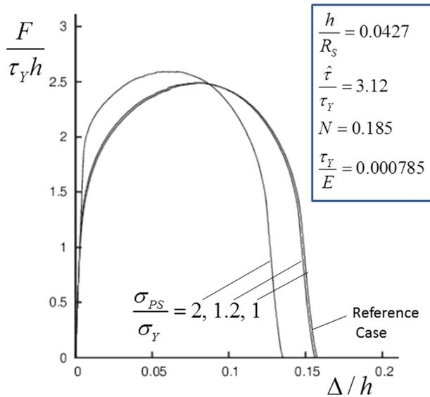
**Fig. 11** A tensile prestress  $\sigma_{PS}$  is applied to the plate to produce uniform plastic stretch and then released prior to cropping. The other dimensionless parameters for the prestress cases (cases 17 and 18) are the same as for case 1, the reference case.
