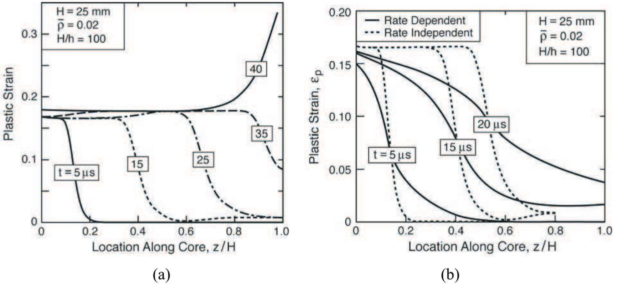
**Figure 12.** Temporal variation in plastic strain distribution calculated for a core without imperfections (to suppress buckling) subject to velocity  $v_0 = 100$  m/s. (a) Rate independent material, and (b) Comparison between rate dependent and rate independent materials.
