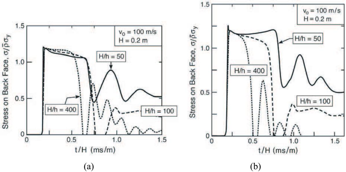
**Figure 17.** The influence of core member slenderness on the stress pulse transmitted through the core. (a) Imperfection amplitude scaled with the member thickness:  $\delta/h = 1$ . (b) Constant imperfection amplitude,  $\delta = 1$  mm.
