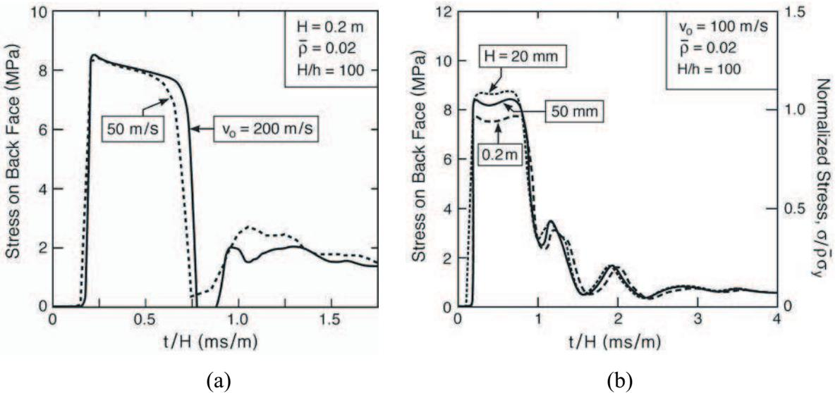
**Figure 16.** The temporal trends in the stress pulse transmitted through the core, with time coordinate normalized by the core height. (a) Effect of imposed velocity at fixed core height. (b) Effects of core height at fixed velocity.
