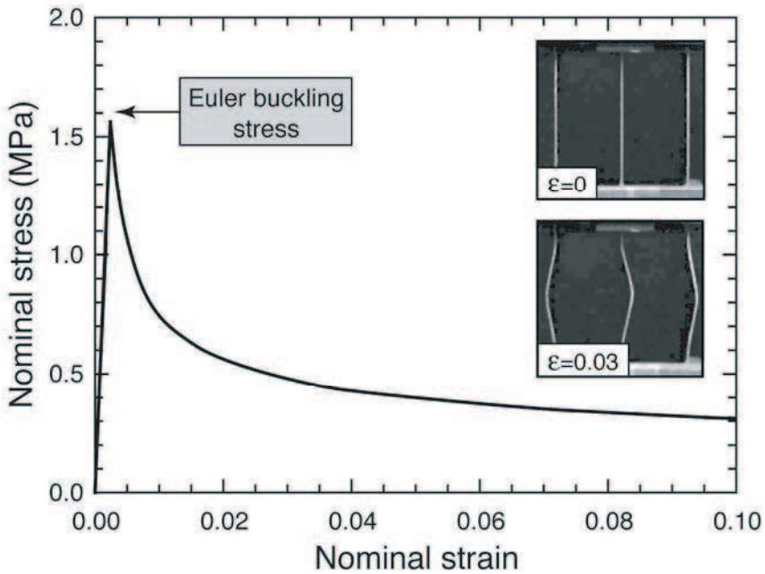
Figure 4. Quasistatic compressive response of I-core specimen.
