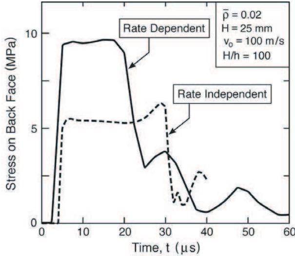
**Figure 15.** The temporal dependence of the stresses induced on the back face when a velocity  $v_0 = 100$  m/s is imposed at one end, including comparison between rate dependent and rate independent materials. Note that the former results in a higher stress but shorter pulse duration.
