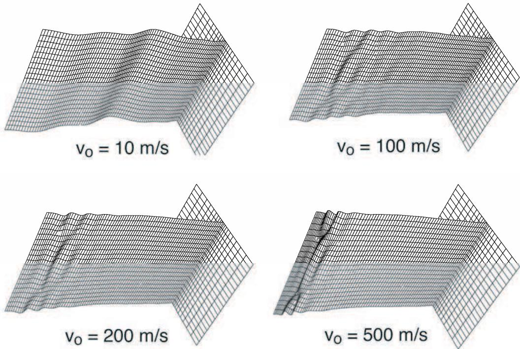
**Figure 11.** Buckle waves induced at several imposed velocities. Note that the wavelengths at the highest velocities are shorter than those of the initial imperfections (Figure 9). ( $H = 25$  mm,  $\bar{\rho} = 0.02$ ).
