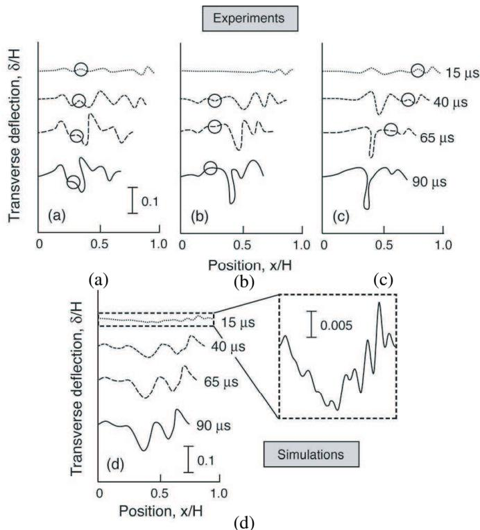
**Figure 6.** (a)–(c) Buckle patterns obtained from high speed photography at imposed velocity  $v_0 = 95$  m/s at several times after impact. The circles show examples of buckles that were well defined in the early stages but were subsequently consumed by the growth of adjacent buckles. (d) Simulations corresponding to experimental measurements. Inset shows detail of the buckle pattern at the earliest time.
