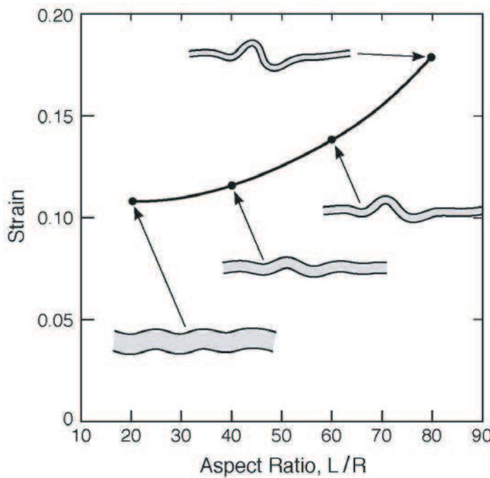
**Figure 1.** Buckle waves generated in free standing slender columns subject to a constant velocity at one end (the left). The plot indicates the terminal value of the nominal plastic strain [Vaughn and Hutchinson 2006].
