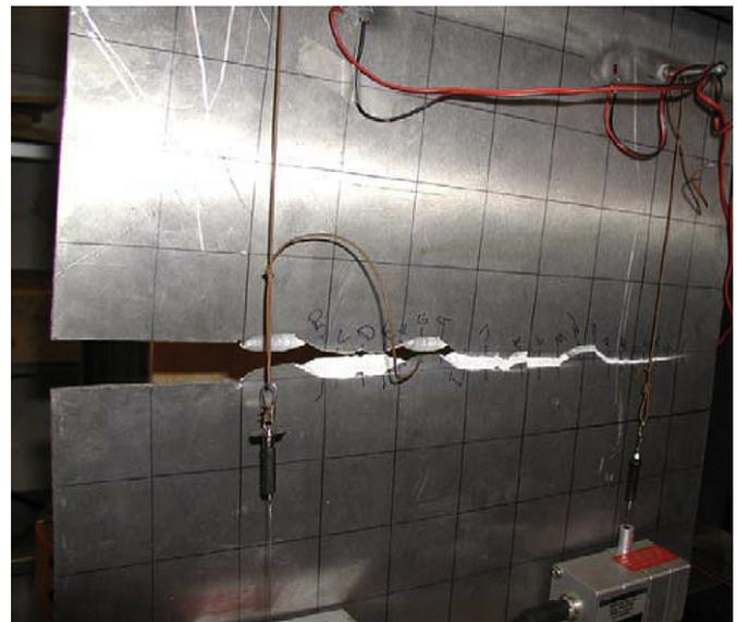
Fig. 2. A 10 mm thick plate of A5083 aluminum tested by Simonsen and Törnqvist [5]. The crack was initiated at the edge notch located on the left edge of the plate. Flipping of the slant fracture from one 45° orientation to the other is evident.
