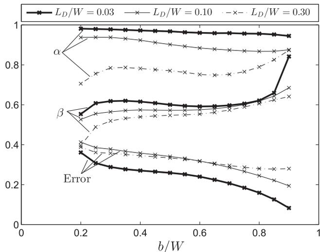
**Fig. 7.** Match between the deformed top surface and the target surface for various indenter widths,  $b/W$ . The match is quantified by the “ $\alpha$ ” and “ $\beta$ ” value specified in Fig. 6, as-well as the  $\text{Error} = \int_0^W |y_{def} - y_{target}| dx / A_{Deformed}$ . Results are shown for  $L_D/W = [0.03, 0.1, 0.3]$ , and  $N = 0.1$  (Case A boundary conditions,  $H/W = 0.5$ , and  $\Delta_0/H = 0.02$ ).
