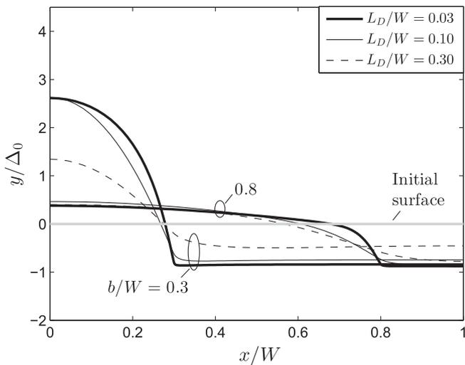
**Fig. 5.** Deformed top surface after unloading the indenter, here displaying the effect of strain gradients. Results are shown for two indenter widths,  $b/W = [0.3, 0.8]$ , and with  $L_D/W = [0.03, 0.1, 0.3]$ , and  $N = 0.1$  (Case A boundary conditions). Here,  $\Delta_0$  is the maximum indentation depth ( $\Delta_0/H = 0.02$  and  $H/W = 0.5$ ).
