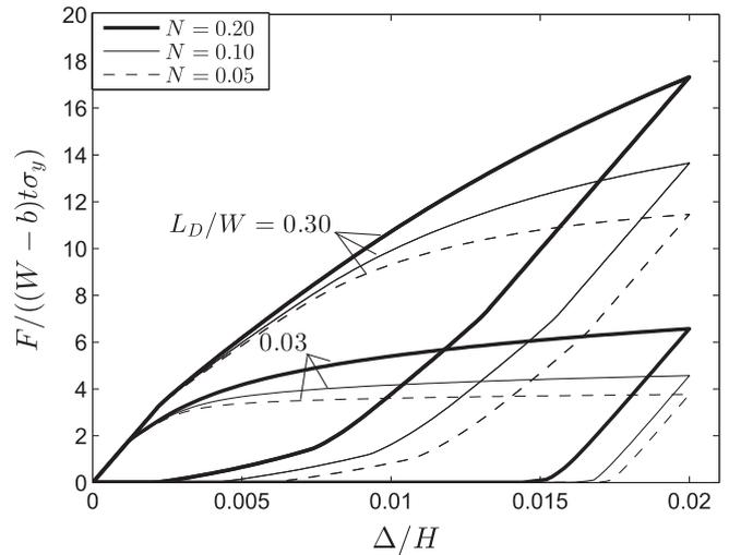
**Fig. 3.** Punch response curves showing the effect of conventional strain hardening and hardening owing to plastic strain gradients. Results are shown for  $L_D/W = [0.03, 0.3], N = [0.05, 0.1, 0.2]$ , and  $b/W = 0.3$  (Case A boundary conditions, and  $H/W = 0.5$ ).
