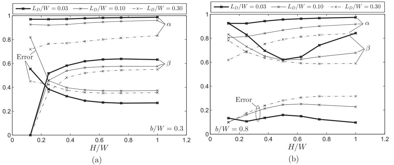
**Fig. 10.** Match between the deformed top surface and the target surface for various sheet thicknesses,  $H/W$ , for two indenter widths; (a)  $b/W = 0.3$ , and (b)  $b/W = 0.8$ . The match is quantified by the “ $\alpha$ ” and “ $\beta$ ” value specified in Fig. 6, as-well as the  $Error = \int_0^W |y_{def} - y_{target}| dx / A_{Deformed}$ . Results are shown for  $L_D/W = [0.03, 0.1, 0.3]$ , and  $N = 0.1$  (Case A boundary conditions, and  $\Delta_0/H = 0.02$ ).
