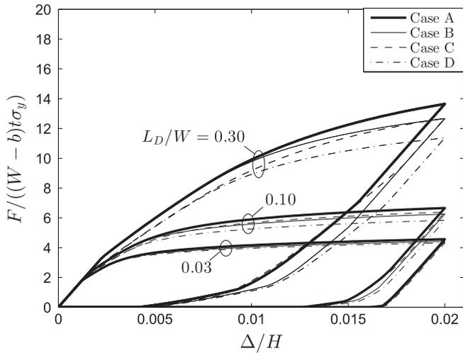
**Fig. 2.** Punch response curves displaying both loading and unloading of the indenter. Results are shown for  $L_D/W = [0.03, 0.1, 0.3]$ , for the four boundary configurations at the indenter interface; Case A ( $\dot{\epsilon}_{ij}^p = 0, \dot{u}_1 = 0$ ), Case B ( $\dot{\epsilon}_{ij}^p = 0, T_1 = 0$ ), Case C ( $t_{ij} = 0, \dot{u}_1 = 0$ ), and Case D ( $t_{ij} = 0, T_1 = 0$ ). Here,  $N = 0.1, b/W = 0.3$ , and  $H/W = 0.5$ .
