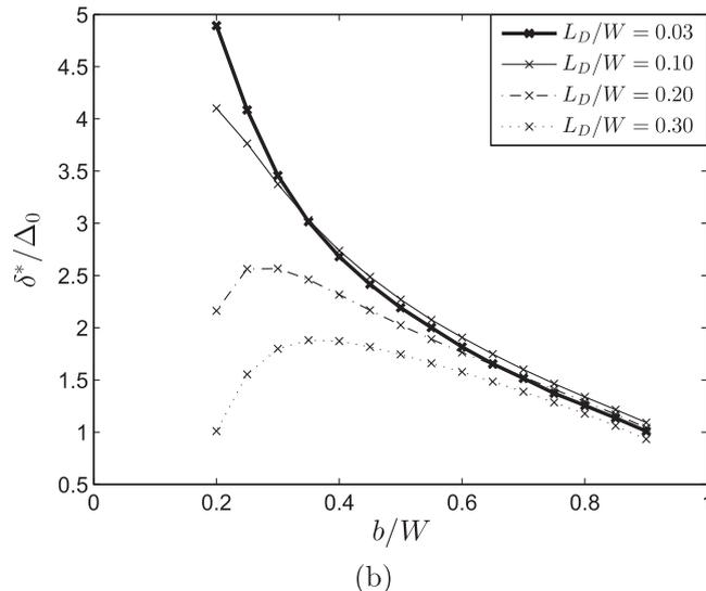
**Fig. 8.** Normalized a) peak load,  $F_{max}$ , and b) maximum indenter depth,  $\delta^*$ , respectively, for various indenter widths,  $b/W$ , and fixed sheet thickness,  $H/W = 0.5$ . Results are shown for  $L_D/W = [0.03, 0.1, 0.2, 0.3]$ , and  $N = 0.1$  (Case A boundary conditions). Here,  $\Delta_0$  is the maximum indentation depth ( $\Delta_0/H = 0.02$ ).
