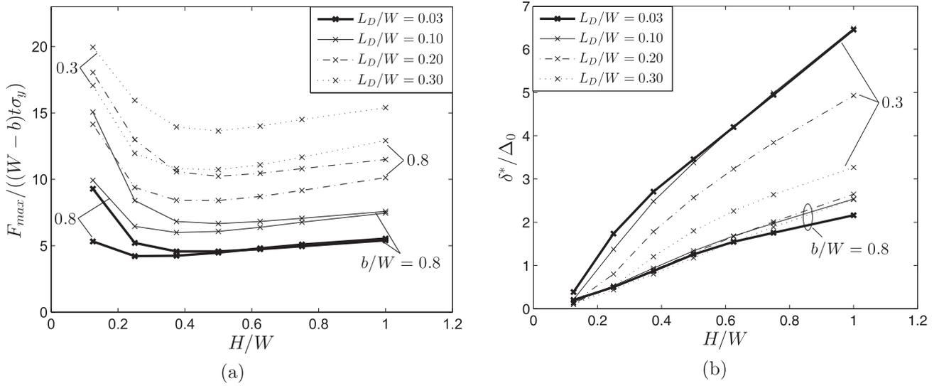
**Fig. 9.** Normalized (a) peak load,  $F_{max}$ , and (b) maximum indenter depth,  $\delta^*$ , respectively, for various sheet thicknesses,  $H/W$ , and fixed indenter width at  $b/W = 0.3$  and  $b/W = 0.8$ , respectively. Results are shown for  $L_D/W = [0.03, 0.1, 0.2, 0.3]$ , and  $N = 0.1$  (Case A boundary conditions). Here,  $\Delta_0$  is the maximum indentation depth ( $\Delta_0/H = 0.02$ ).
