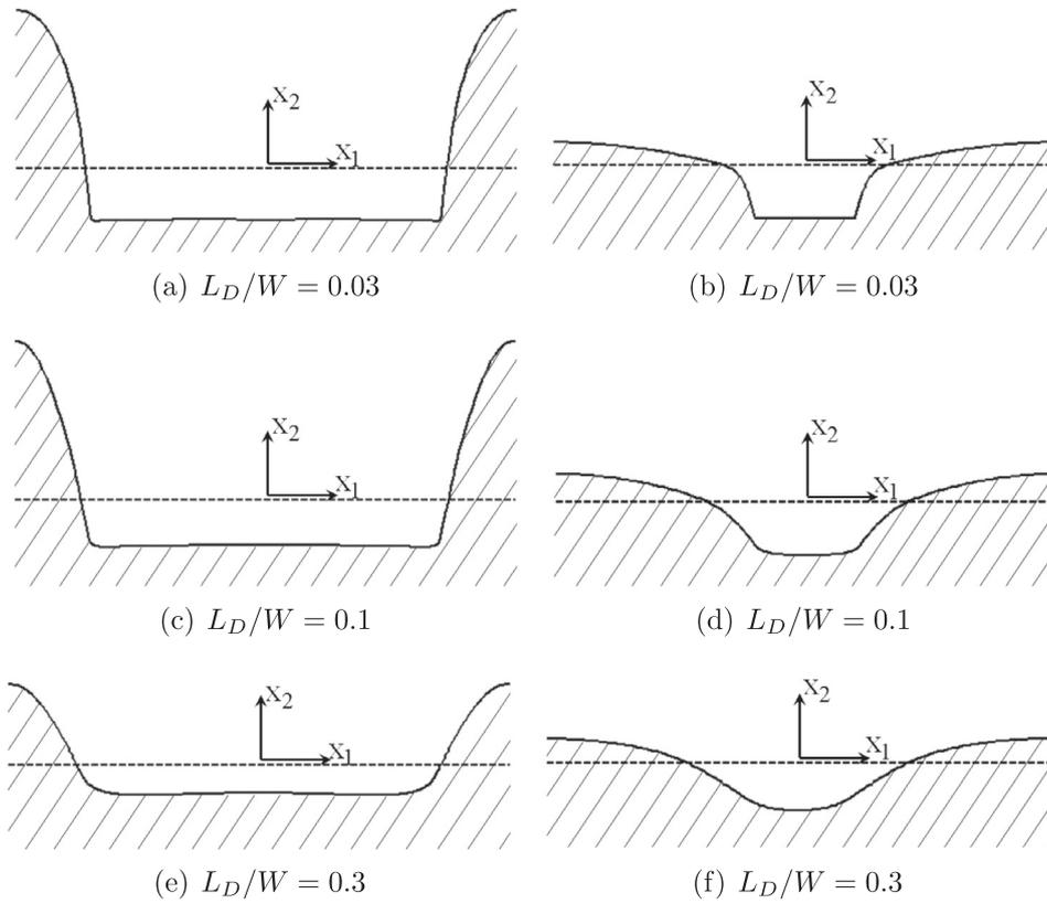
**Fig. 4.** Deformed top surface after unloading the indenter, where the hatched area indicates the gradient enhanced solid and the dashed line indicates the initial top surface. Results are shown for two indenter widths,  $b/W = [0.3, 0.8]$ , with  $L_D/W = [0.03, 0.1, 0.3]$ , and  $N = 0.1$  (Case A boundary conditions). Here,  $\Delta_0$  is the maximum indentation depth ( $\Delta_0/H = 0.02$  and  $H/W = 0.5$ ).
