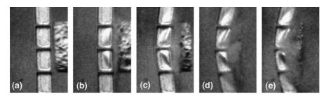
Fig. 12. A photographic sequence showing crushing of the foam projectile and deformation of the sandwich beam. The image in (a) was taken immediately before impact; the subsequent images were taken at 40 μs intervals. The impact velocity was 330 m/s.
