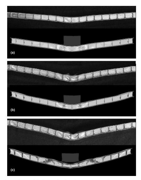
Fig. 6. Representative sandwich beams following dynamic testing, at impulse levels: (a) 2.7, (b) 3.8 and (c) 4.6 kPa s. The first image in each pair is a photograph of the actual test specimen; the second is from the finite element simulation.
