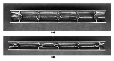
Fig. 11. Cross-sections through specimens tested in quasi-static compression at plastic strains of (a) 0.16 and (b) 0.47. Note the symmetry of each buckled core member.
