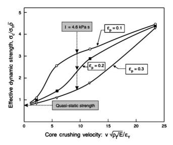
Fig. 15. Calculated effect of core crushing velocity on the effective dynamic strength. The velocity acquired at the highest impulse is superposed. Here  $\bar{\rho}$ ,  $\rho_f$ , E and  $\varepsilon_y$  are the core relative density, the mass density of the solid material, the Young's modulus and the yield strain, respectively.
