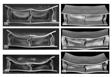
Fig. 10. Transverse cross-sections showing core crushing at impact sites, at impulse levels (a) 3.3, (b) 3.8 and (c) 4.6 kPa s. The sequence in (d)–(f) shows the corresponding finite element predictions at the same impulse levels.
