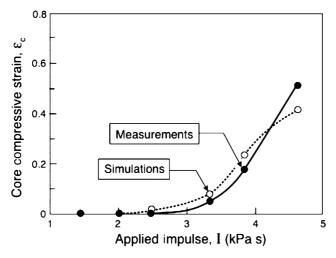
Fig. 9. Core compressive strain in sandwich beams at impact site.
