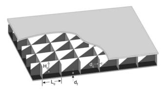
Fig. 4. Honeycomb-core sandwich geometry.
