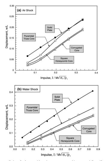
Fig. 1. Synopsis of deflection predictions for beams with various core types, subject to spatially uniform impulse (a) in air and (b) under water. Here, M is the mass per unit area of the beam.
