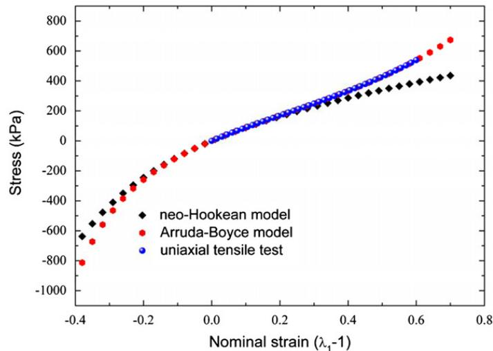
**Fig. 2.** Tensile stress–strain data of the PDMS used in the present experiments and the tensile predictions for the neo-Hookean model and the Arruda–Boyce model. The two constitutive models are taken to be incompressible and have been fit to a ground state shear modulus, 0.32 MPa. The locking parameter of the Arruda–Boyce model has been taken as  $\lambda_m=1.17$ .
