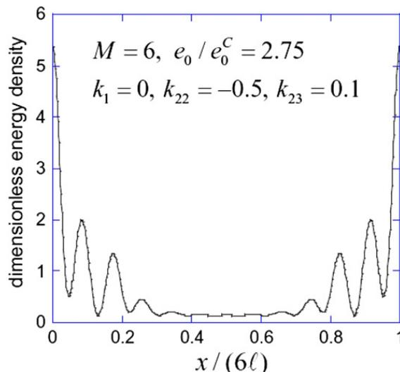
**Fig. 14.** Distribution of the dimensionless energy density of the film/substrate system (the integrand of (4.8)) for one of the fully nonlinear solutions in Fig. 12. This plot reveals the highly localized nature of the deformation in the vicinity of the ridges.
