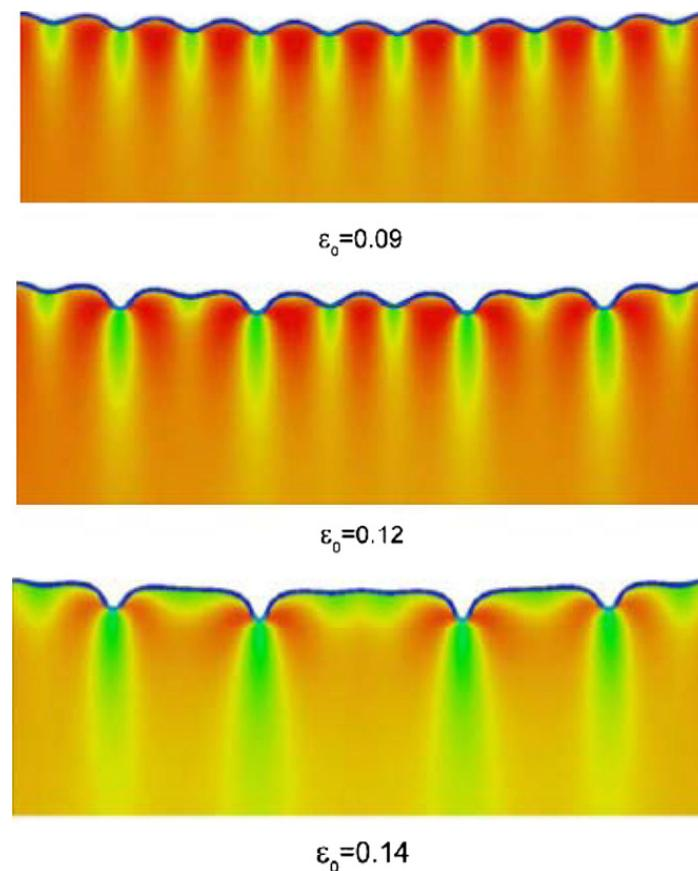
**Fig. 6.** A sequence of wrinkle patterns showing the emergence of period-doubling followed by developing folds. The film and the substrate are modeled by the Arruda–Boyce model with the substrate fit to the data in Fig. 2 for PDMS. The film/substrate modulus ratio is  $\mu_f/\mu_s = 100$ . The substrate is pre-compressed to  $\lambda_1^S = 0.7$  prior to attachment of the film and subsequent to imposition of the overall compressive strain  $\varepsilon_0$ .
