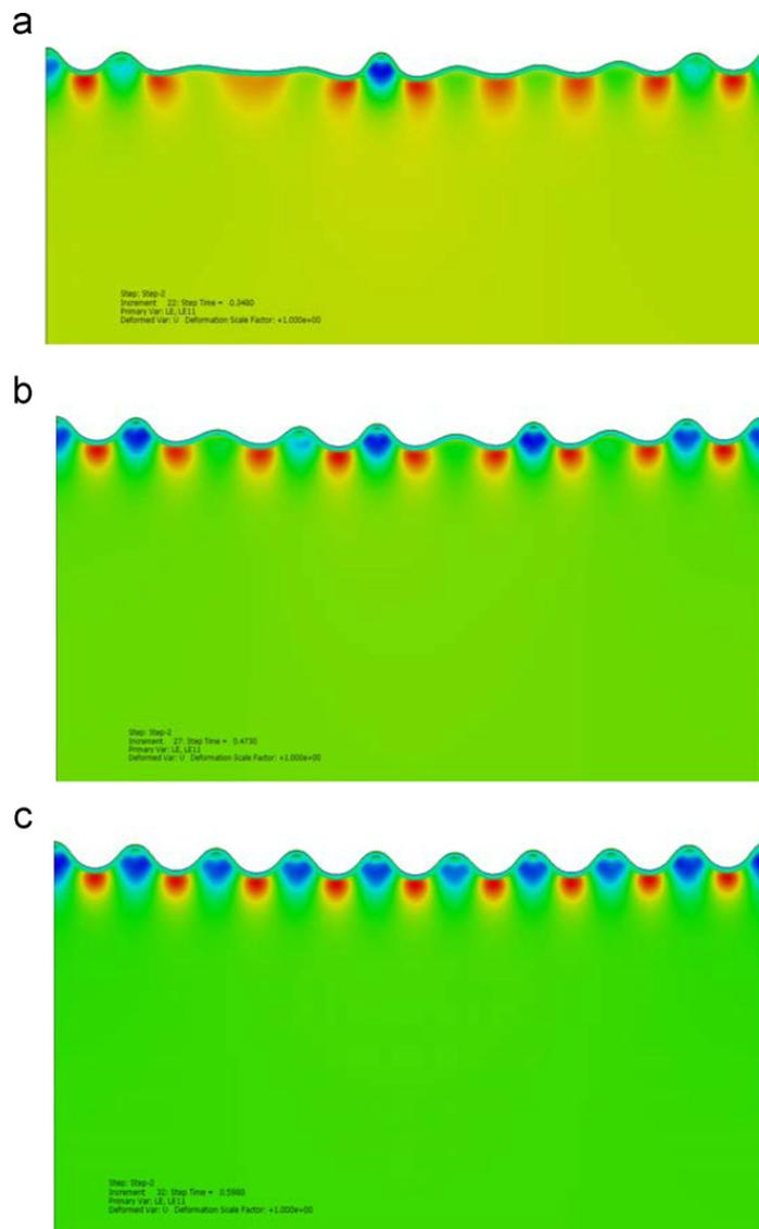
**Fig. 5.** Sequence of wrinkle patterns for an Arruda–Boyce film/substrate system with  $\mu_f/\mu_s=100$  and a substrate pre-stretch  $\lambda_1^S=1.5$ . The simulation reveals that the ridge mode reverts back to the periodic sinusoidal mode as the compression is increased. Both the film and substrate are taken to be incompressible with locking parameter  $\lambda_m=1.17$ . (a) Overall strain  $\varepsilon_0=0.115$ , (b)  $\varepsilon_0=0.16$ , (c)  $\varepsilon_0=0.20$ .
