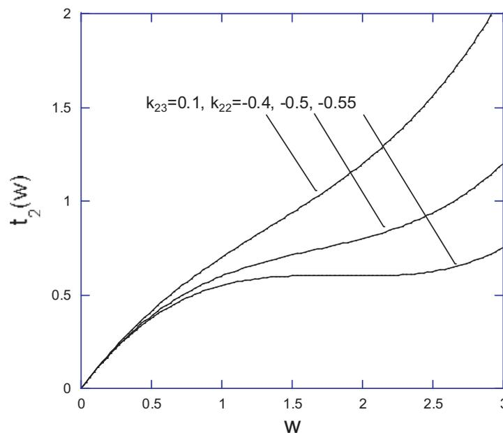
**Fig. 8.** An illustration of the dimensionless nonlinear normal traction–displacement relation with nonlinearity qualitatively representative of a substrate that has experienced pre-stretch (compare with Fig. 7). The curve with  $k_{22} = -0.5$  and  $k_{23} = 0.1$  will be used in the simulations based on the one-dimensional model.
