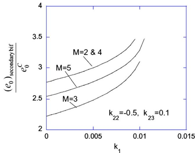
Fig. 10. The overall compressive strain associated with secondary bifurcation from the primary solution for secondary modes with periodic wavelengths,  $M\ell$ . The lowest strain for secondary bifurcation is associated with modes having  $M=3$ . An example of a secondary mode shape is given in Fig. 11. Secondary bifurcations with periodicities that are integer multiples of  $\ell$  do not occur for  $k_1$  greater than about 0.01.
