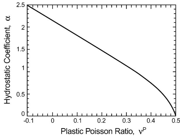
Fig. 3. The dependence of the hydrostatic coefficient  $\alpha$  on the plastic Poisson ratio,  $v^p$ .
