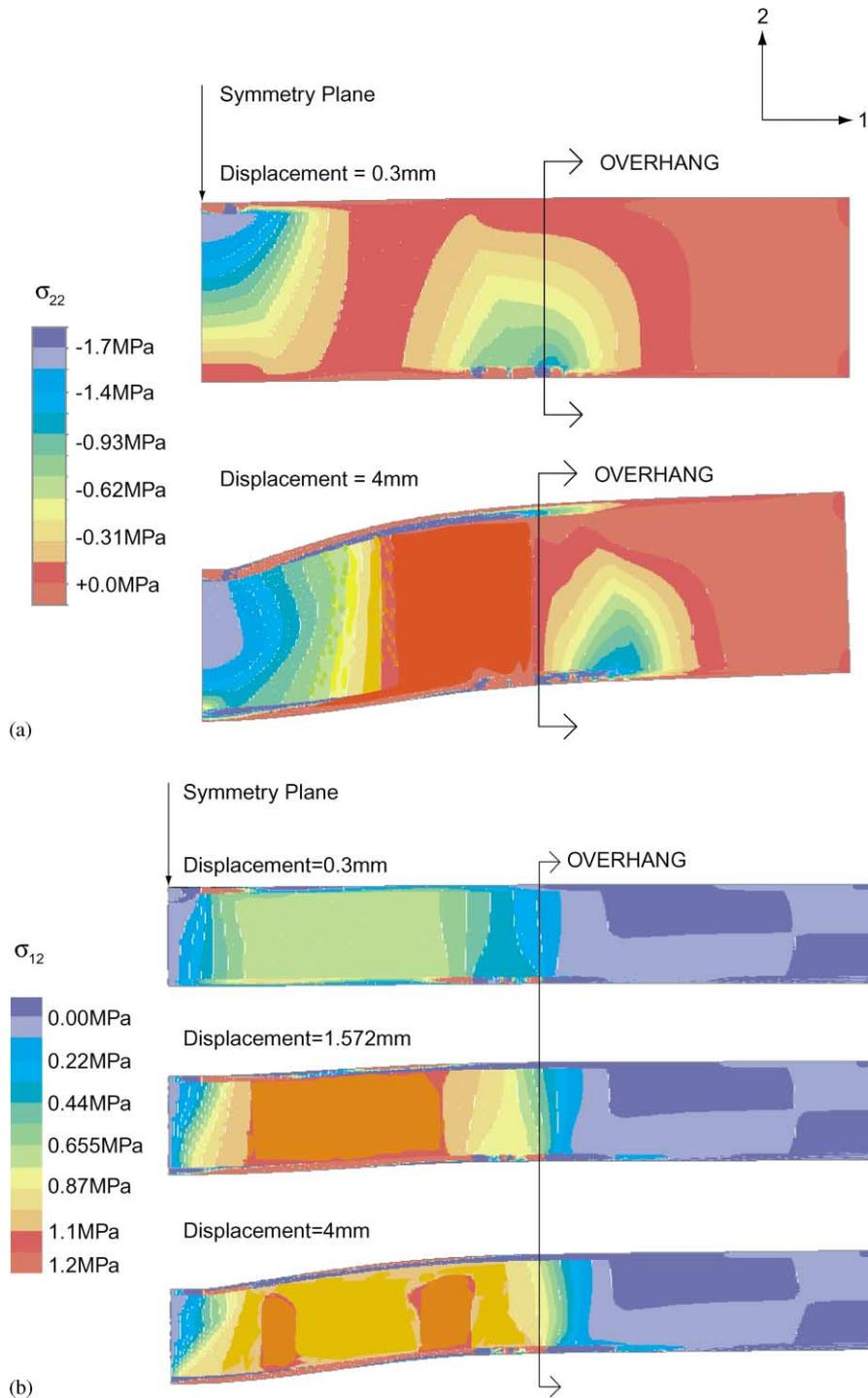
Fig. 9. Finite element results showing the stress distributions. (a) Specimen that fails by indentation. Notice the significant plastic deformation within the bottom face sheet in addition to indentation by the loading fixture. (b) Specimen that fails by core shear. Notice the shear deformation of the core within the overhang.
