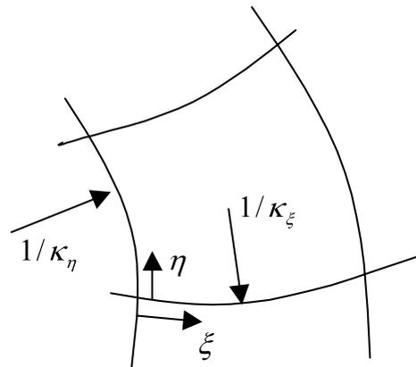
Fig. 1. Curvilinear slip line field.
