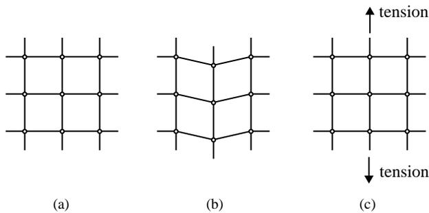
Fig. 2. (a) An infinite repetitive square grid structure showing; (b) one possible mechanism; and (c) one possible state of self-stress.
