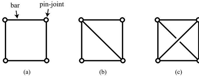
Fig. 1. (a) A kinematically indeterminate structure, with one mechanism, (b) a statically and kinematically determinate structure and (c) a statically indeterminate structure, with one state of self-stress.
