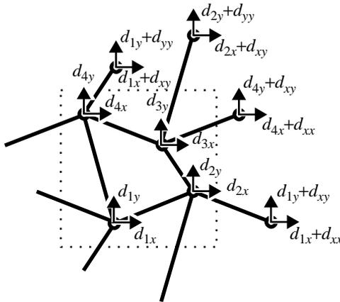
Fig. 7. An augmented nodal displacement numbering scheme for the perturbed square grid, allowing displacements of the nodes ( $d_{1x}$ – $d_{4y}$ ) and deformation of the unit cell ( $d_{xx}$ ,  $d_{yy}$ ,  $d_{xy}$ ).
