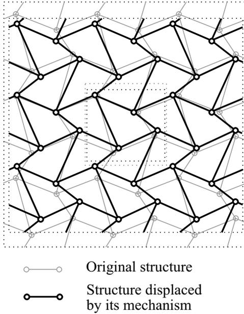
Fig. 6. The mechanism of the perturbed grid shown in Fig. 4; note the deformation of the unit cell.
