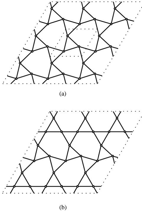
Fig. 5. Two mechanisms of the kagome structure: (a) the finite mechanism; and (b) one possible infinitesimal mechanism.
